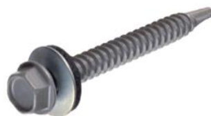
#14 x 1 1/2" T-5 Self-drilling, Fenderhead Dyna-Coat Coated HWH Screw with EPDM Washer
