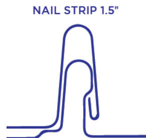
Figure 7. Compatible Panel Seams – PV Cube KLOC
